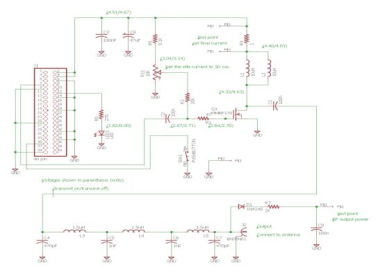
Figure 1: WSPR Transmitter Schematic
